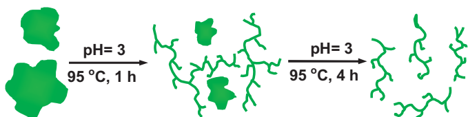
Fig. 3. Hydrolysis process scheme for the preparation of hydrolyzed peach gum polysaccharide (HPGP) from CPG.
